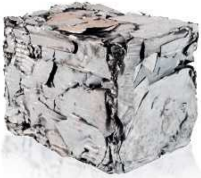
A scrap cube measures 50 cm along the edges and weighs 200 kg. Up to 4 000 scrap bales a day are processed at the foundry; they contain many valuable raw materials.
